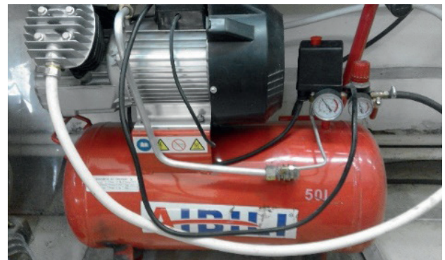
Figure 2. Device for removing dust from core cavities
